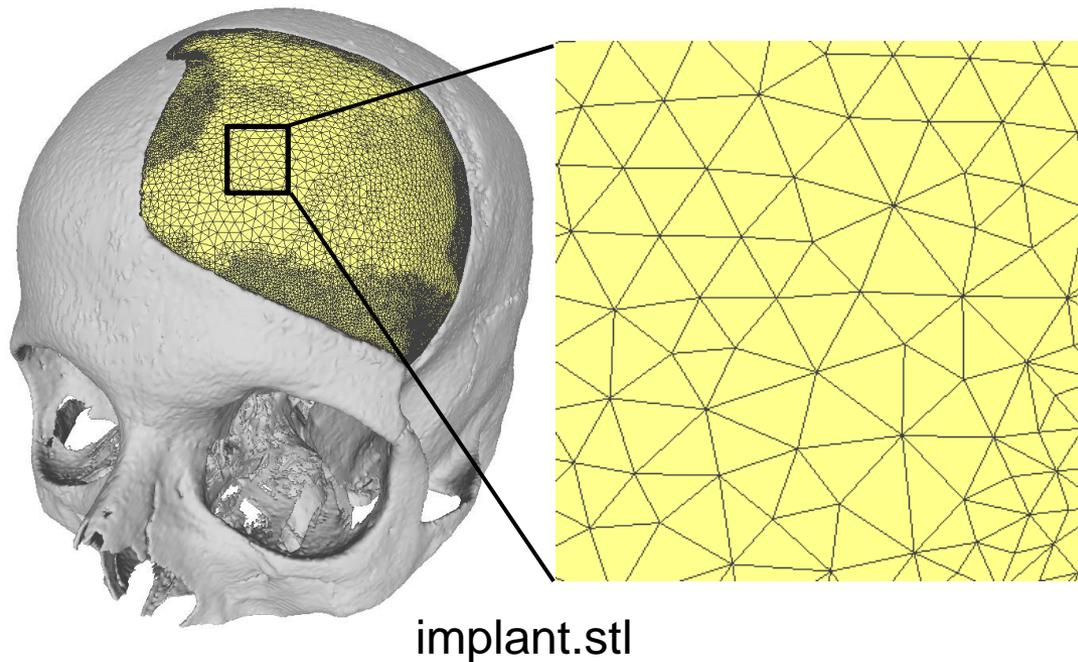
.stl files describe the surface geometry of a 3D model (e.g., an implant) using triangular meshes
